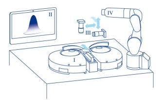
Fig. 3 Schematic design: positioning system for fine adjustment (I), application-specific software and user interface (II), industrial image processing (III) and conventional robotics for pick-andplace of the components (IV) (image: PI)
