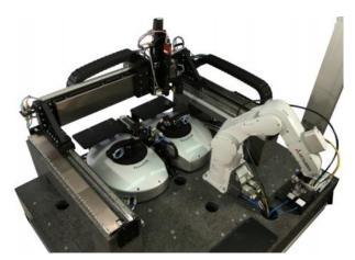
Fig. 1 Automated solution for silicon photonic chip production and inspection: the system integrates several hardware components and software for the automation of assembly and alignment, such as pick-and-place robot technology, image processing, or devices for precision positioning (image: PI)
