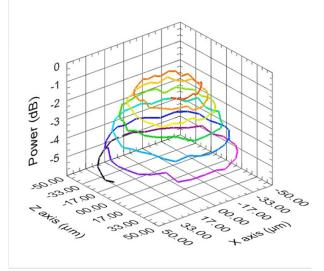
Fig. 5 Fine adjustment for fiber array. The light throughput is measured and optimized via scan algorithms (image: PI)
