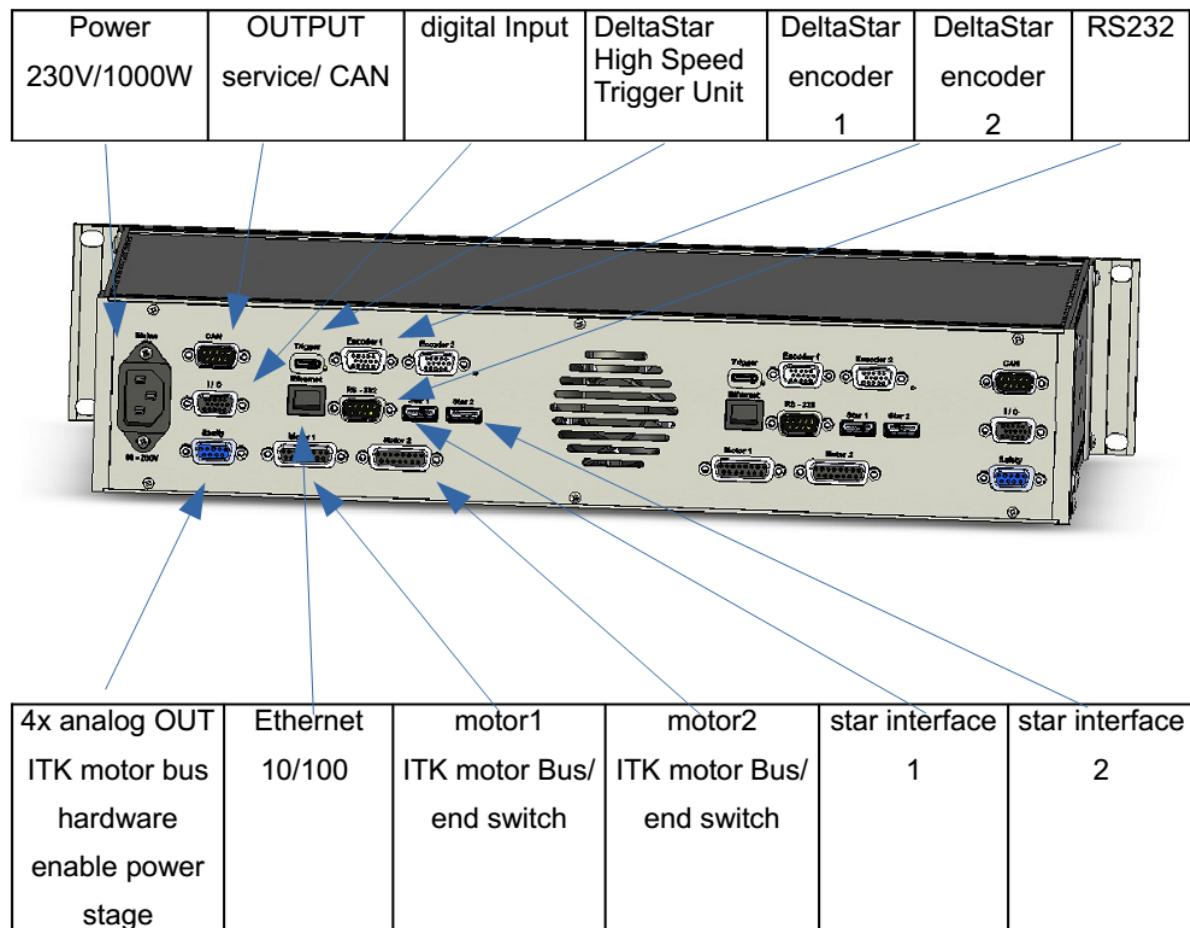
According to the previous pages, please connect the stages to the controller. The controller is completely configured for the system.
