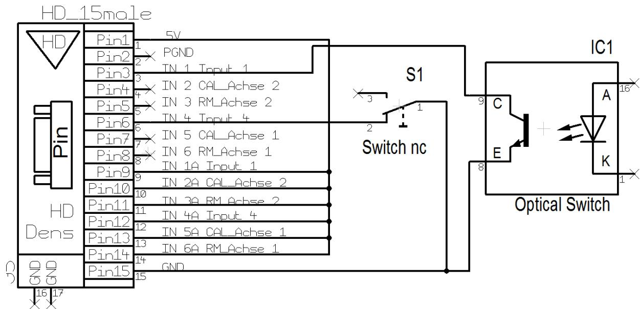
If the external sensor is a different type or should be galvanically isolated, we need to disconnect the reference Pins IN-1A and IN-4A and do a new connection to the reference-voltage of the external supply.
